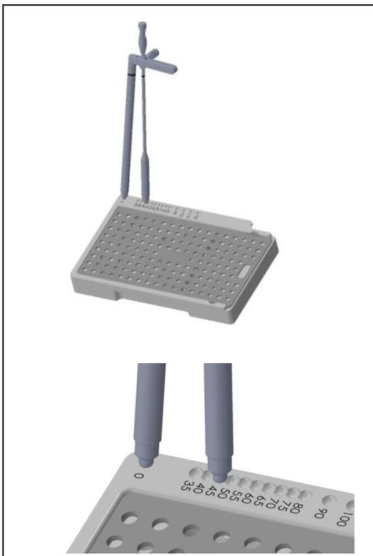
Take the locked calipers to the rod caddy of choice (either straight or curved) and place the end of one caliper arm into the dimple labeled zero. Allow the other arm to fall into whichever corresponding length dimple it aligns with.
