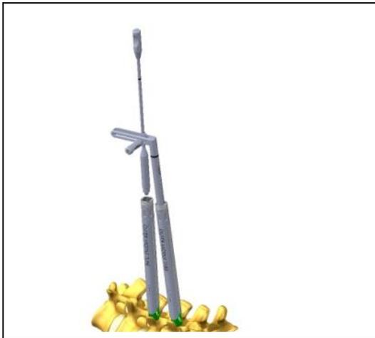
Lock the caliper arms by tightening the nut at the top of the calipers.
