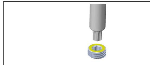
Place a set screw on the end of the tightener, making sure the gold side of the set screw is facing up along the shaft of the tightener.
