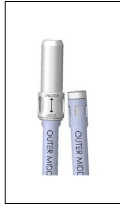
If more than 25mm of reduction is required, the **threaded reduction caps** may be used. Each cap can be placed onto a tube assembly by pulling up on the outer collar of the cap and then pushing the cap down onto the top of the tube assembly. Each cap has three prongs that are designed to seat into one of the six oval windows at the top of the tube assembly.
