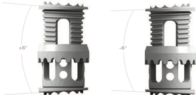
**Figure 4: The end caps can be rotated 180° to reconstruct either a thoracic kyphotic or a lumbar lordotic curve. Above example uses two 3° end caps.**
