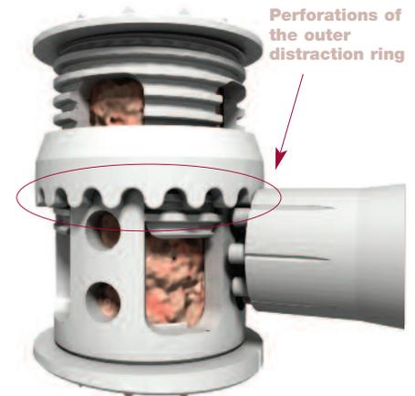
Figure 27: Placement of the perforated tips of the outer cannulated shaft of the expander in between the scallops of the outer distraction ring.
