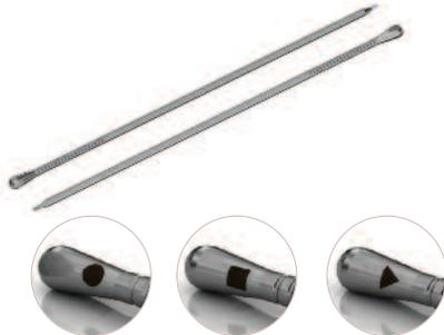
The VLIFT implant contains a pre-assembled locking screw, which is locked with the screwdriver to secure the implant height after distraction. The screwdriver is placed into the head of the locking screw *in situ*, which is then turned (backed-out) two full turns counterclockwise to lock the distraction mechanism in place.
