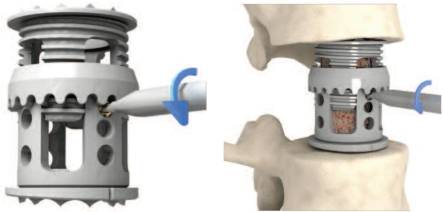
**Figure 34:** The screwdriver engages the pre-assembled locking screw. Two counterclockwise turns of the locking screw with the screwdriver will lock the implant height in place.
